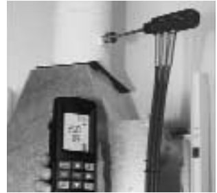
CO measurement up to 4000 ppm
